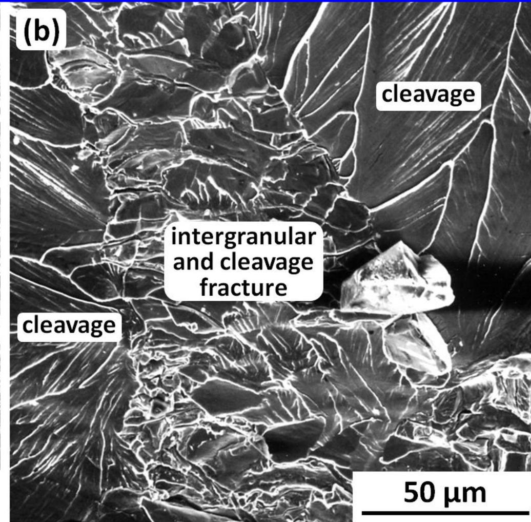
● Brittle fracture: cleavage of coarse grains and intergranular + cleavage fracture of fine grains.
