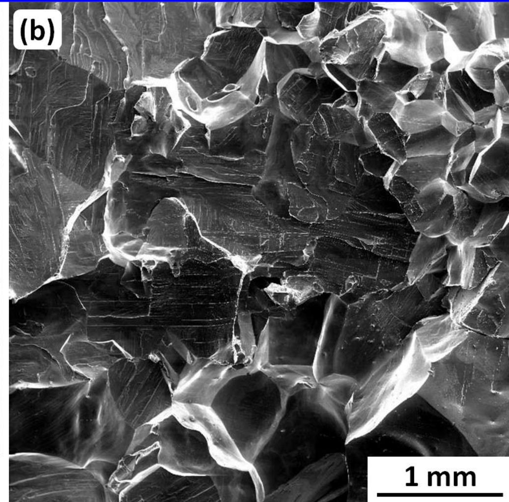
● Brittle fracture: (a) Near-surface: intergranular; (b) interior: intergranular + cleavage.
