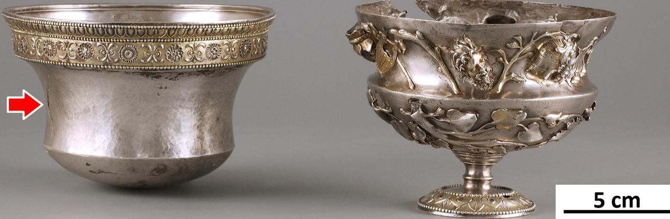
recrystallized surface grains owing to final planishing + annealing
