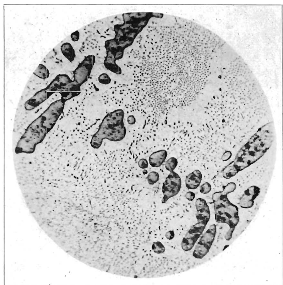
FIG. 2.—BADLY OXIDIZED COPPER, SHOWING OXIDE CRYSTALS AND EUTECTIC, UN- ETCHED. × 200.
