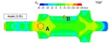
Qualifying RS at location A is inferred based on measured data at location B, and computed relationship between A and B
