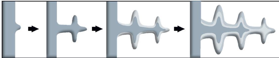
*Schematic of dendritic microsegregation (coring) during dendrite formation*
