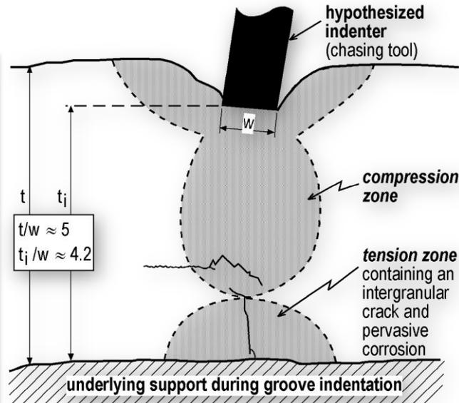
*schematic suggests a deformation “pattern” from the slip-line field theory of indentation: the theory predicts a tension zone opposite the indented (chased) groove when  $t_i/w = 4.4$  (close to actual value)*
