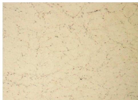
SPEE3D heat treated microstructure
