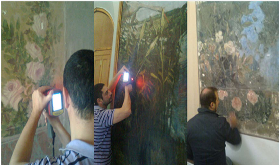
Images: Colleague Eng. Aguilera measuring chemical composition with the Portable XRF on the walls of the Fader Museum and the Curator indicating better places to do measurings.
