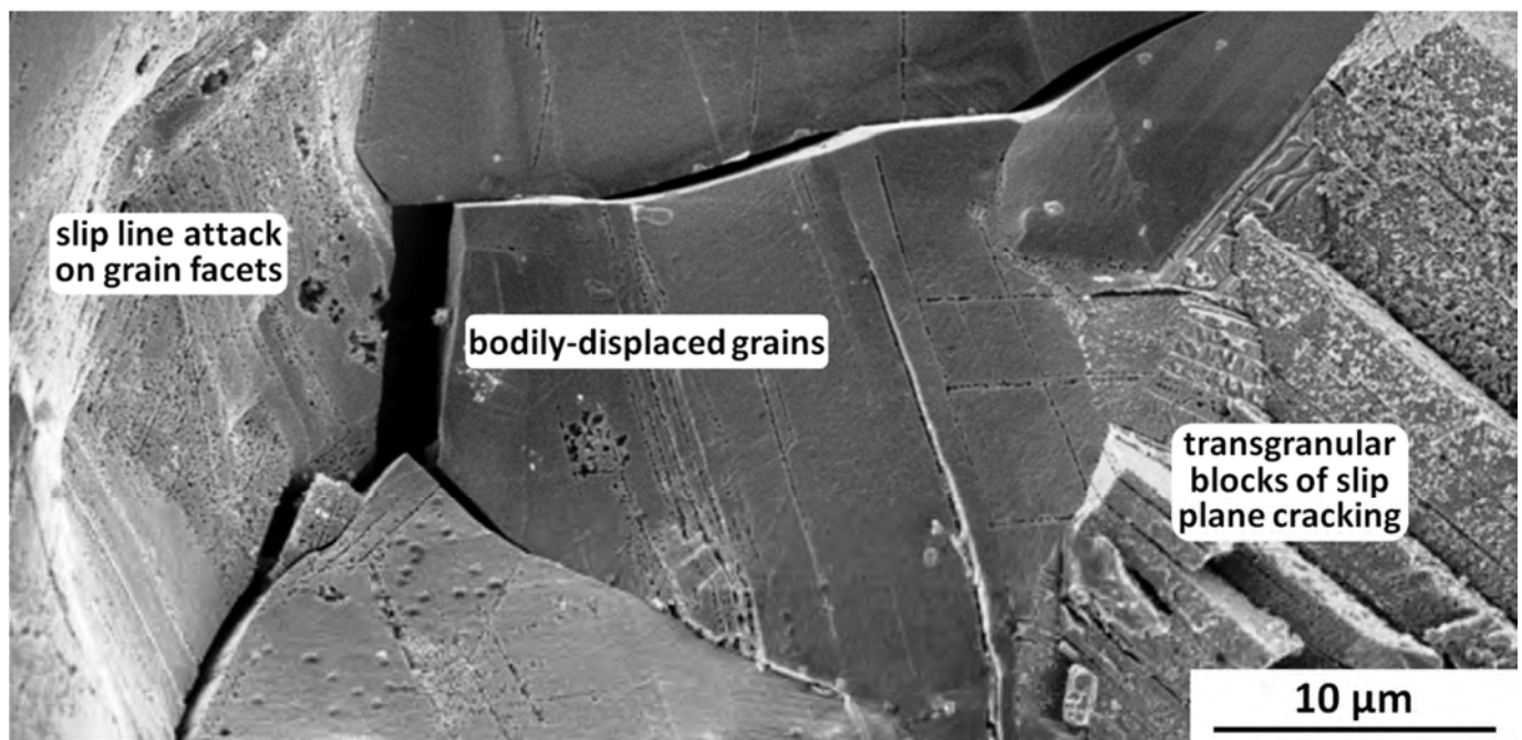
Figure 20. Example SEM SE fractograph for the Egyptian Vase showing (i) bodily displaced grains and consequently widened cracks diagnostic for microstructural embrittlement, (ii) slip line attack and transgranular blocks of slip plane cracking diagnostic for SCC of cold-worked high-silver artifacts. Original image with permission: Tim Hattenberg, Netherlands Aerospace Centre, Marknesse, the Netherlands.
