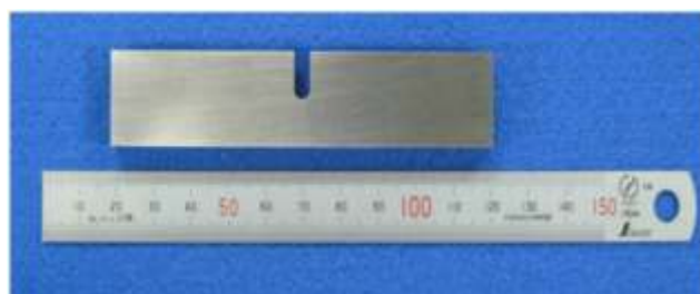
Fig. 1 Photograph of the (a) Three Point Bend Specimen and (b) Specimen setup in autoclave with ACPD connection.
